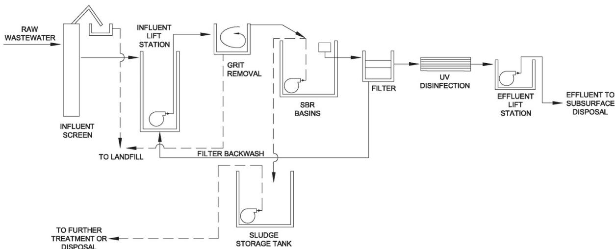
An SBR was chosen for the Class A treatment because it has a smaller footprint than a conventional activated sludge system or oxidation ditch, both of which require secondary clarifiers. This smaller footprint may work well for the limited space available in each community. The SBR also requires less maintenance and operational expertise than a membrane bioreactor system (MBR). The treatment system is estimated to be a Class 3 system according to OAR-049-0020.
