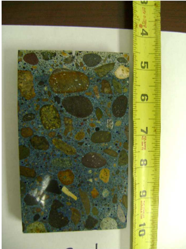
Photograph #1 - Sample 06033-1. Change in paste color can be seen at top surface and lower right corner.
