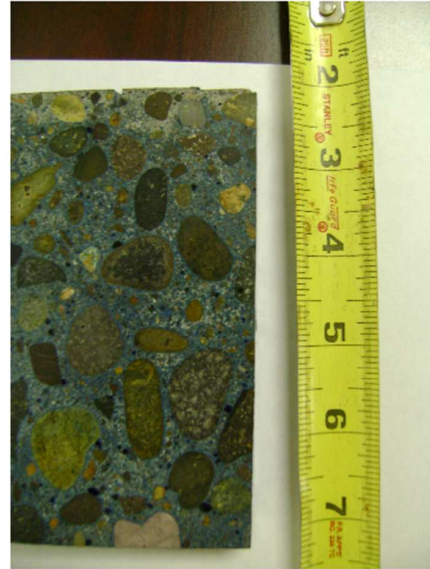
Photograph #2 - Sample 06033-2. Color change can be seen in paste at top surface as well as the bulk paste.
