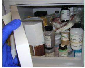
Inadequate storage cabinets and excess volume can lead to stacking glass bottles filled with chemicals and leaking containers that obscure labels. This creates a risk of incompatible chemicals mixing and leaking chemicals coming in contact with science teachers reaching into the cabinet.
