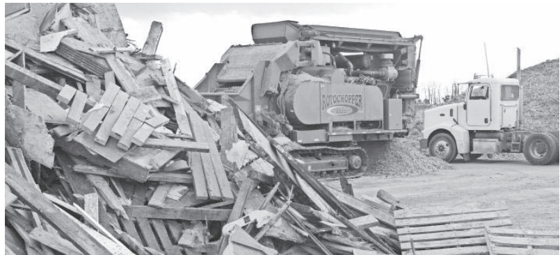
Used construction wood is ground up as hog fuel to be converted into boilers to produce energy. SPECIAL TO THE STATESMAN JOURNAL
