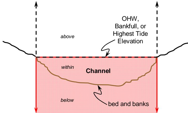
Figure 6. Channel conditions and/or clear span determine whether the Stream Simulation *active channel width* (ACW) criterium is met. The bridge in this diagram meets the Stream Simulation ACW criterium for both channel cases.
