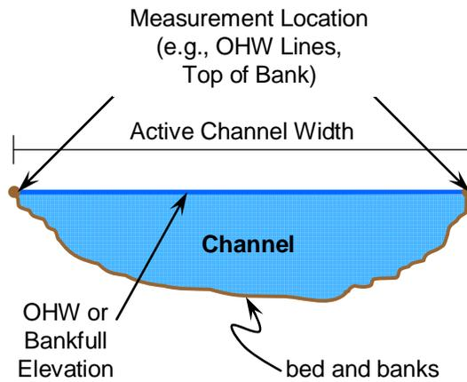
Figure 2. Delineation of a channel.
