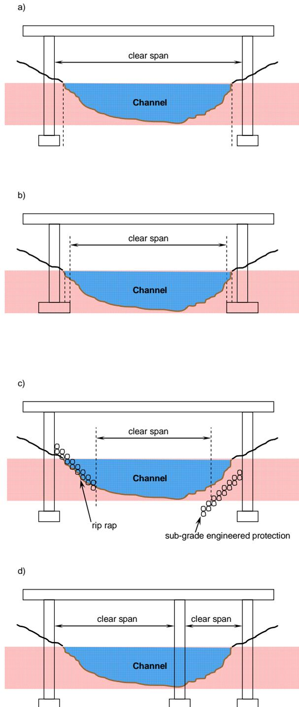
Figure 5. Zones relevant to bridge triggers. Presence of *bridge elements* in the "shaded zone" (i.e., within or below the *channel*) determines whether a trigger is possible. All (and only) *bridge elements* in the vertical plane of the *channel* (i.e., within, below, and above) should be considered for the 50% measure of whether repair/maintenance/modification of an existing *bridge* is a trigger.
