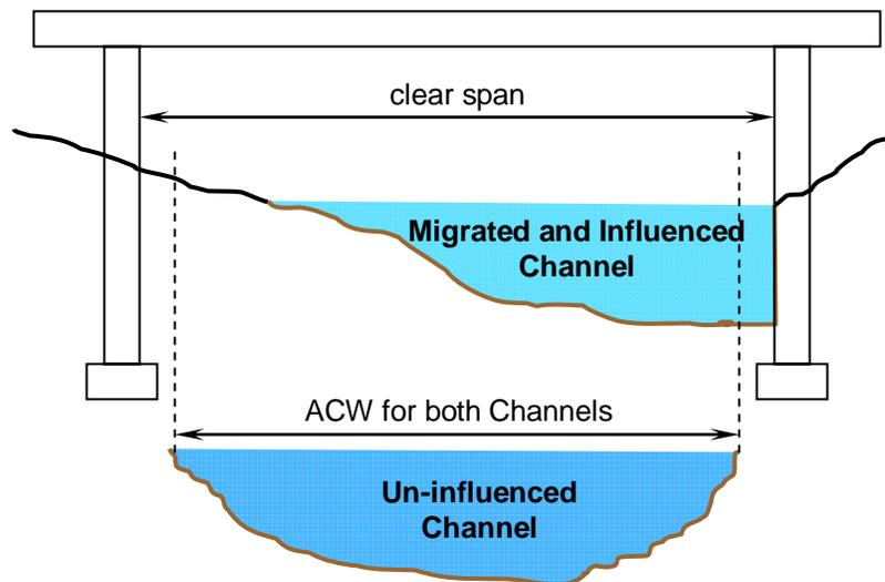
Figure 7. Examples of measurements for Larger-Scale Crossing Guidelines. Note that *active channel width* (ACW) fill is measured at the OHW or bankfull elevation. Anything that replaces or is placed on the *bed and banks* counts toward filled *bed and banks* (e.g., rip rap, exposed footers, poured concrete scour protection).
