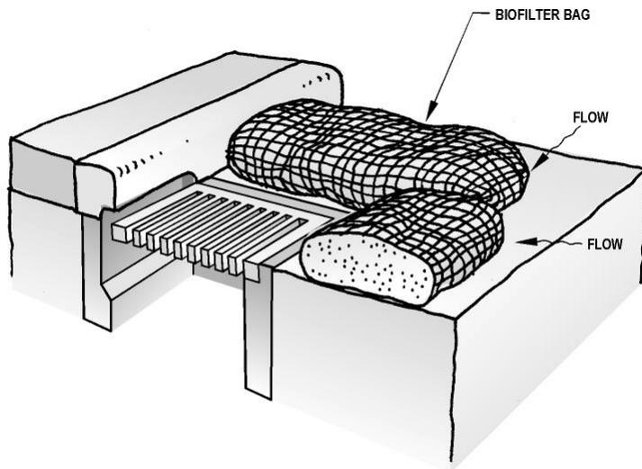
Inlet Protection – Biofilter Bags Around Catch Basin
