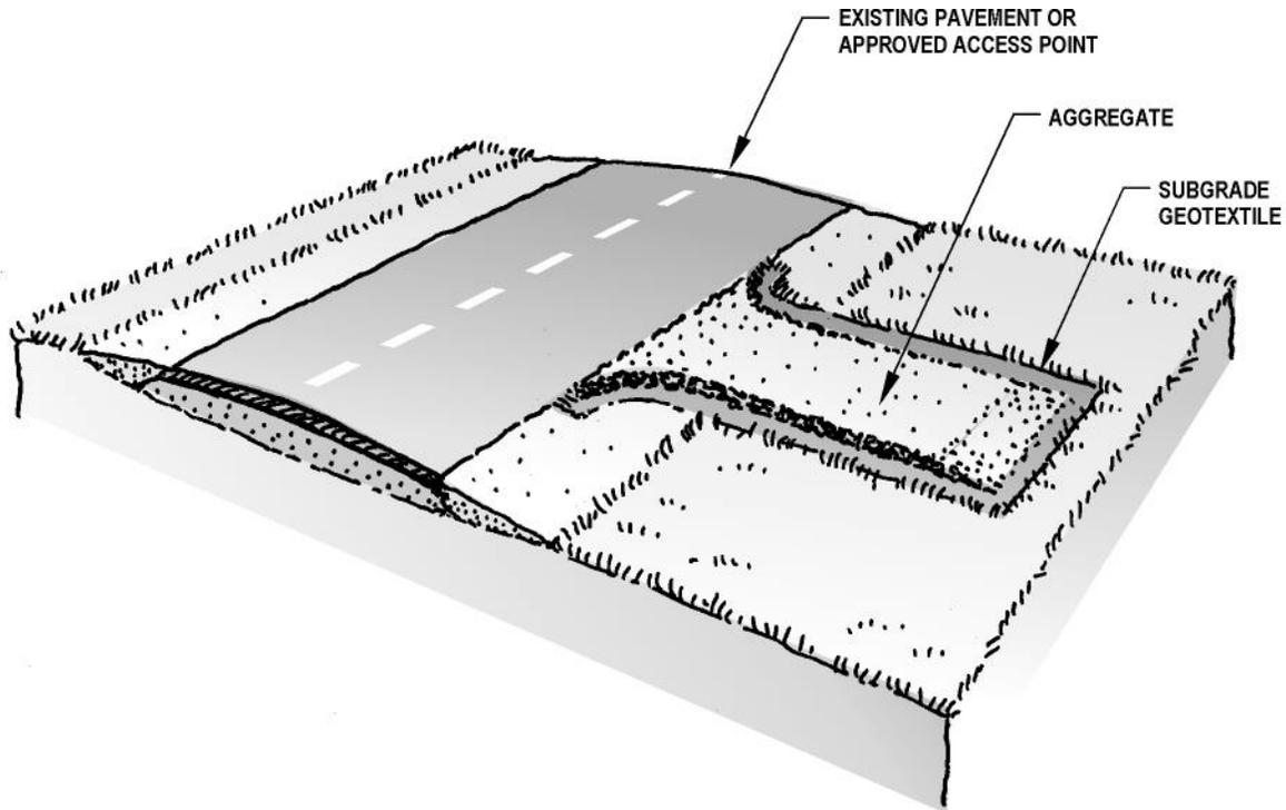
A construction entrance is a stabilized rock pad, placed at construction site ingress/egress locations to reduce the amount of sediment transported onto paved roads by vehicles or runoff. The construction entrance may also include a curb ramp designed out of wood.
