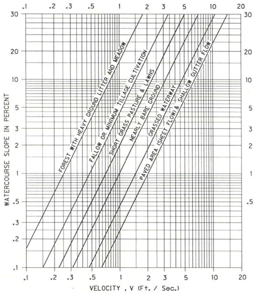
Figure 4-1. Average Velocity of Shallow Concentrated Flow
