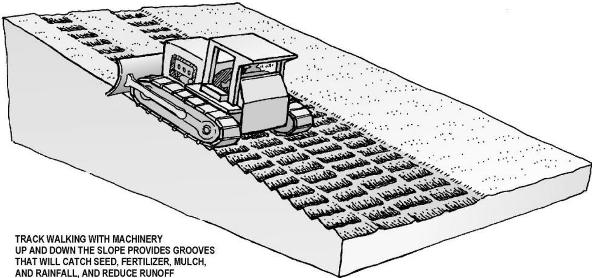
Surface roughening leaves the slopes in a roughened condition after clearing or creating a rough soil surface with horizontal depressions or grooves intended to trap seed and reduce runoff velocity. Roughening can be accomplished by ‘track walking’ slopes with tracked equipment, by using a serrated wing blade attached to the side of a bulldozer, or by other agricultural equipment.
