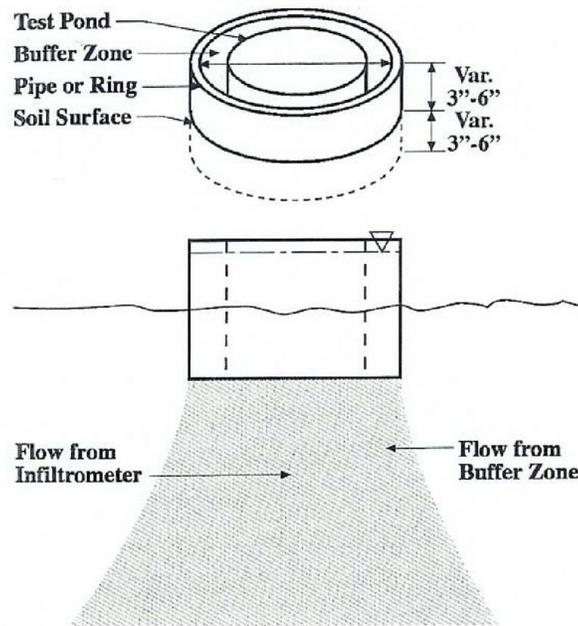
Figure B-2. Double Ring Infiltrometer Test Procedure
