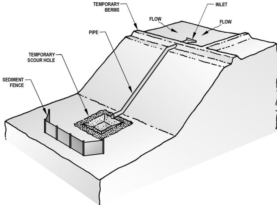
A pipe slope drain is a pipe extending from the top to the bottom of a cut or fill and discharging into a stabilized watercourse, a sediment trapping device or onto a stabilized vegetated area. The pipe slope drain carries concentrated runoff down steep slopes without causing gullies, erosion, or saturation of slide-prone soils.
