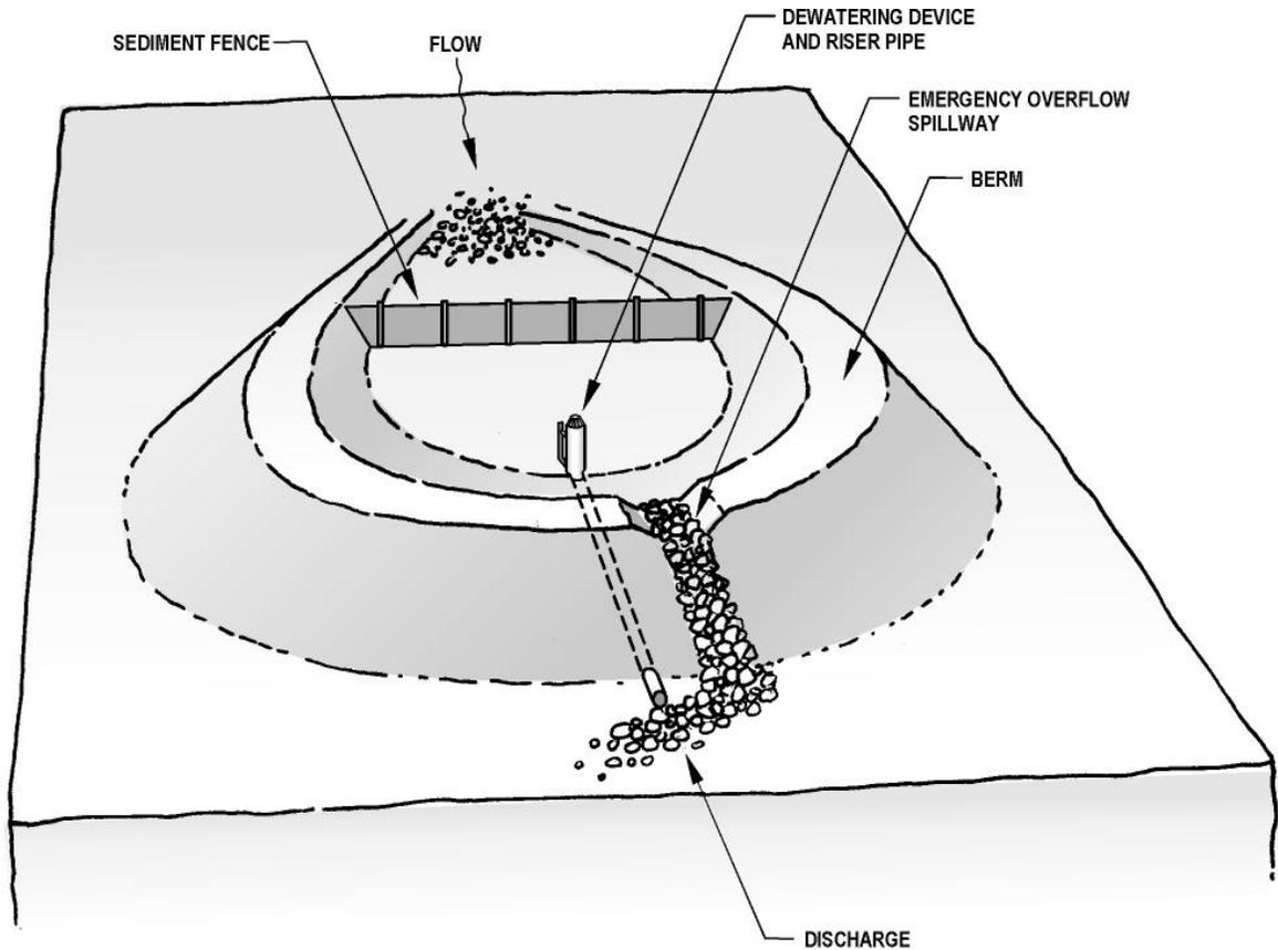
A temporary sediment basin has one or more inflow points and baffles to spread the flow, wet storage and dry storage, a securely anchored riser pipe, a dewatering device and an emergency overflow spillway. A sediment basin should serve a drainage area less than 10 acres in size and have a design life of approximately 1-year.
