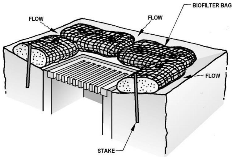
Inlet Protection – Biofilter Bags around Area Drain
