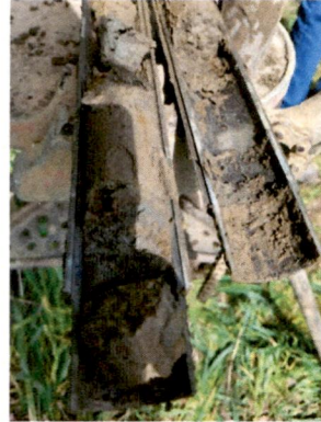
Split Spoon Sample, B-1-16, Depth = 22 feet, OLD FIELD FILL (4/21/2025)
