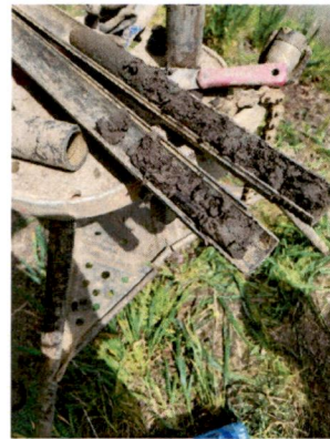
Split Spoon Sample, B-1-19, Depth = 26.5 feet, OLD FIELD FILL
