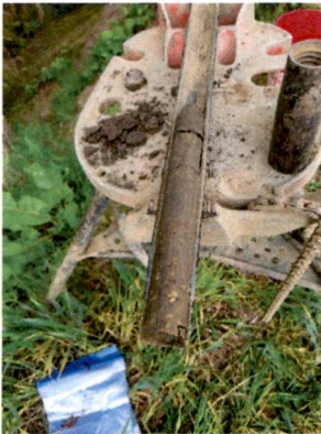
Split Spoon Sample, B-1-5, Depth = 6 feet NEW BERM FILL (4/21/2025)
