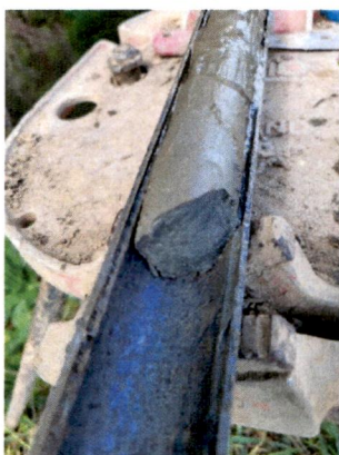
Split Spoon Sample, B-1-22, Depth = 31 feet, Missoula Flood Deposit (4/21/2025)
