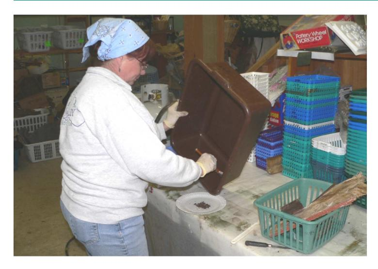
Recovering and weighing dirt from a lumber sample
