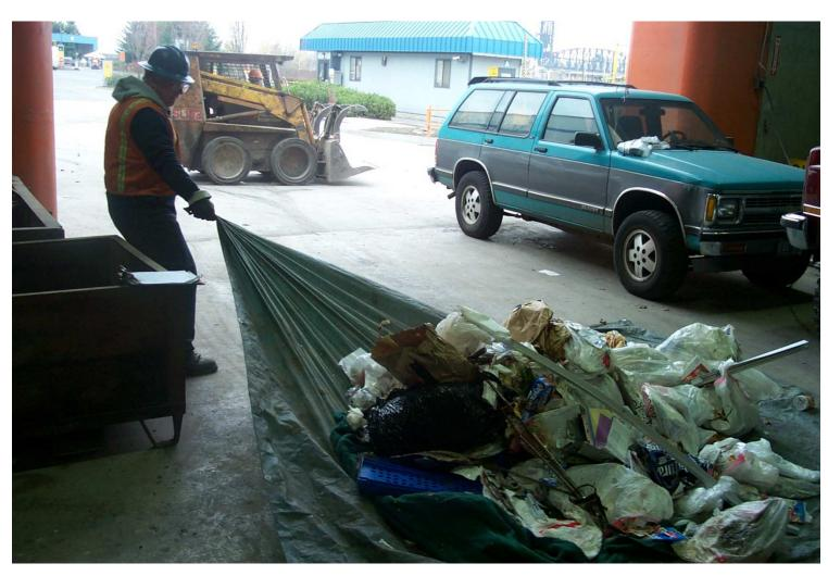
Roughly checking the sample weight. Loads must average 200 lbs or more, and minimum weight is 175 lbs.
