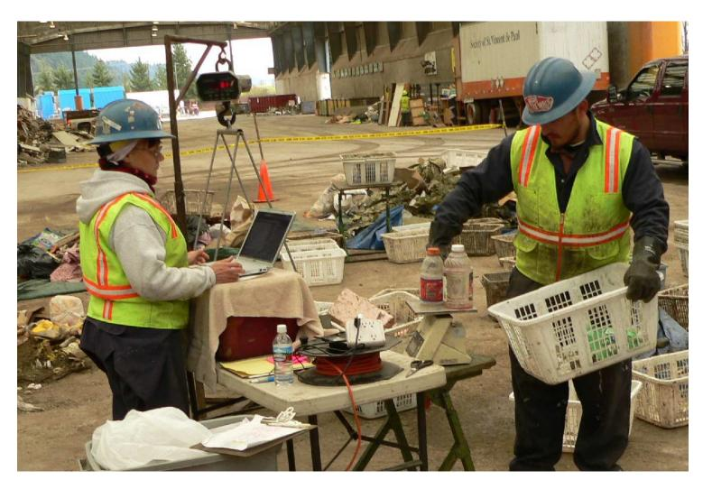
A small scale measuring to 1/100 lbs is used for small items. Beverage containers were also counted.
