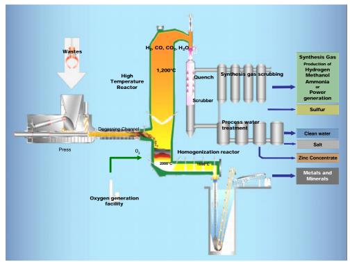
Figure 7- Typical Gasification System<sup>10</sup>
