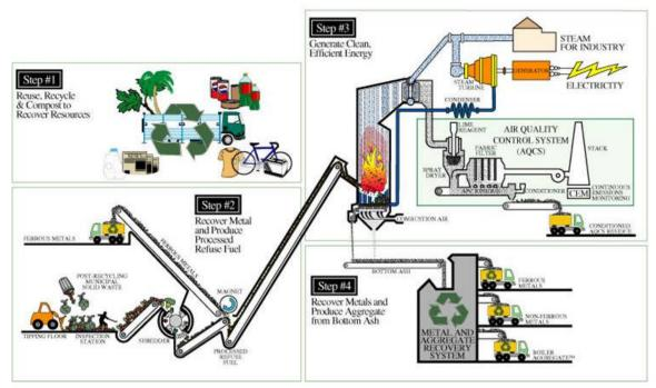
Figure 4 - Typical RDF Combustion Facility<sup>7</sup>
