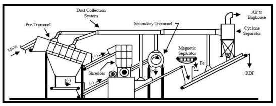
Figure 5 - Typical RDF Processing Schematic<sup>8</sup>
