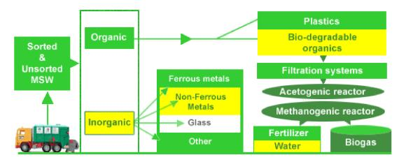
Figure 13 - Process Flow for Anaerobic Digestion System<sup>17</sup>
