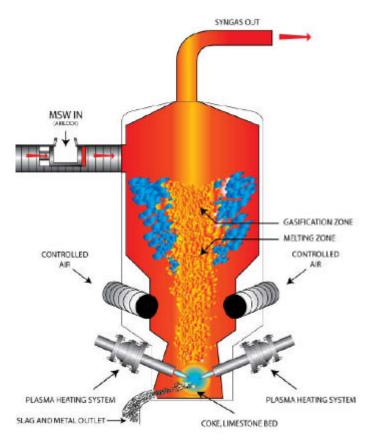
Figure 11 - Cross-Section of a Plasma Arc Furnace<sup>14</sup>
