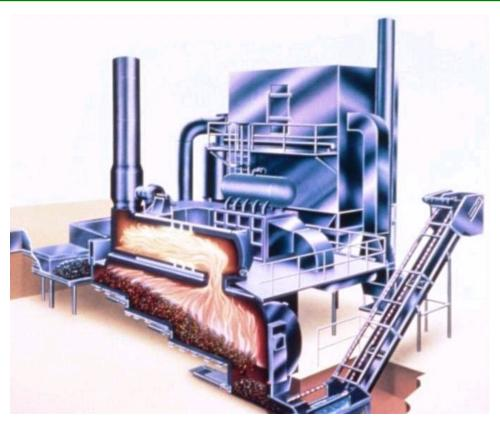
Figure 3 - Typical Modular Combustion System<sup>6</sup>
