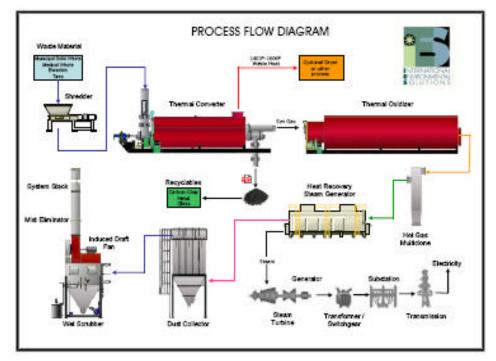
Figure 10 - Process Diagram of a Pyrolysis System<sup>13</sup>
