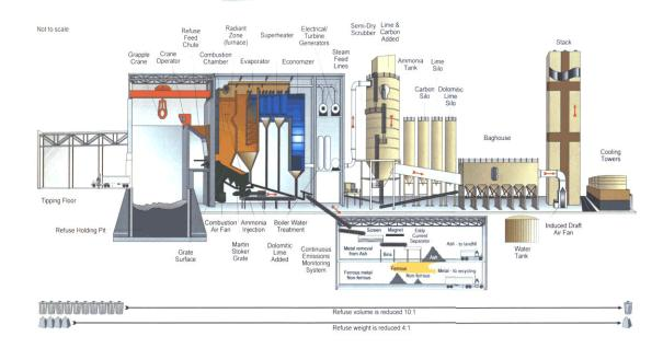
Figure 2 - Typical Mass-Burn Waterwall System<sup>5</sup>
