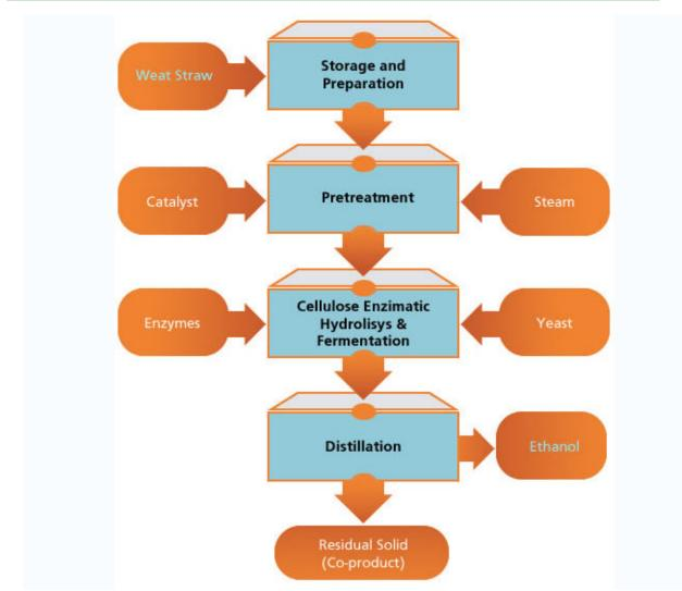
Figure 12 - Process Flow of the BCyL Biomass Ethanol Plant<sup>15</sup>
