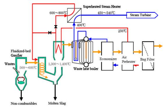
Figure 8 - RDF Fluidized Bed Gasification System<sup>11</sup>
