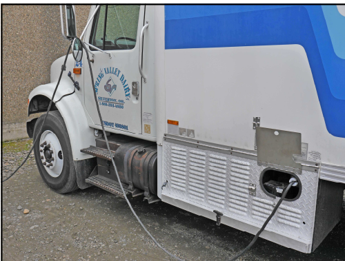
By plugging Spring Valley’s refrigerated trucks up to an electrical source instead of letting them idle, they save over 2,500 gallons of diesel fuel each year.
