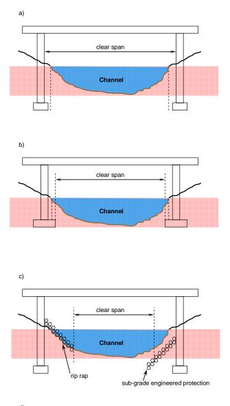
d) clear span cl Figure 5. Zones relevant to bridge triggers. Presence of *bridge elements* in the "shaded zone" (i.e., within or below the *channel*) determines whether a trigger is possible. All (and only) *bridge elements* in the vertical plane of the *channel* (i.e., within, below, and above) should be considered for the 50% measure of whether repair/maintenance/modification of an existing *bridge* is a trigger.
