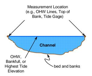
Figure 3. The horizontal plane of the channel (shaded).
