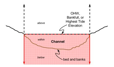
Figure 6. Channel conditions and/or clear span determine whether the Stream Simulation *active channel width* (ACW) criterium is met. The bridge in this diagram meets the Stream Simulation ACW criterium for both channel cases.
