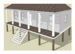
Marion County requires new homes be elevated to 2 feet above the Base Flood Elevation while the State of Oregon minimum is 1 foot. Besides better ensuring homes are kept out of harms way, this additional foot of elevation brings significant savings for property owners on their flood insurance premiums.\*
